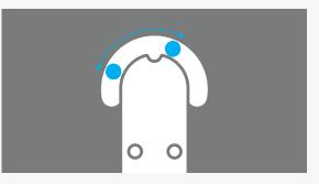
Before bending, the D.I.Wire needs to go through the homing sequence to ensure the bend pin is in the proper position.
